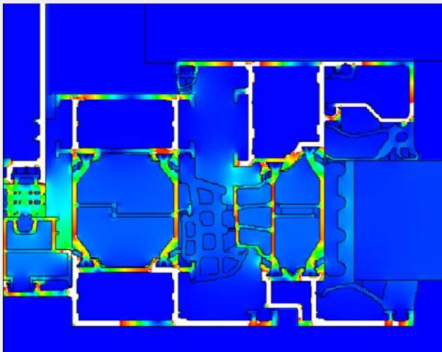
Fig. 22.1: Heat flow - insert window without ALPET®
